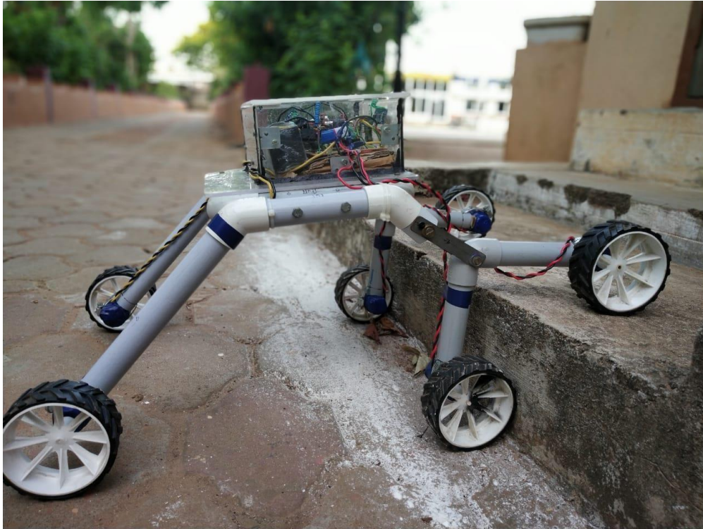
Fig 3.3 – Prototype image showing Rocker Bogie Mechanism
