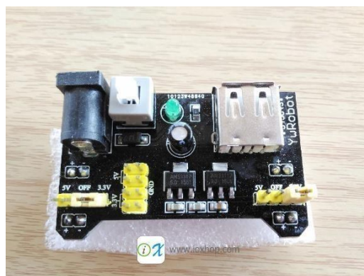
Fig 5.12 – HW-131 Power Distributer
